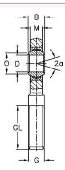
$\begin{array}{lll} A & = 112 \\ a \ (degrees) & = 6 \\ B & = 35 \\ D & = 50 \\ Dynamic \ drive \ (kN) = 308 \\ F & = 185 \\ g & = M45x3 \\ GL & = 107 \\ \end{array}$
